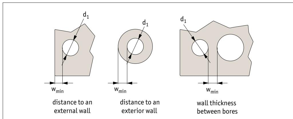
The guidelines for minimum wall thickness or distance from an edge ( $w_{\min}$ ) are shown below – these minimum values produce only a very slight deformation on the exterior profile (less than 20 microns).
