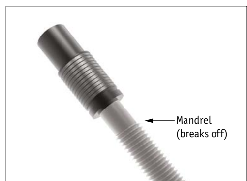
“Pull” Expansion sealing plugs. Pulling on the mandrel expands the sleeve, sealing the channel. At a predetermined force the mandrel breaks off.
